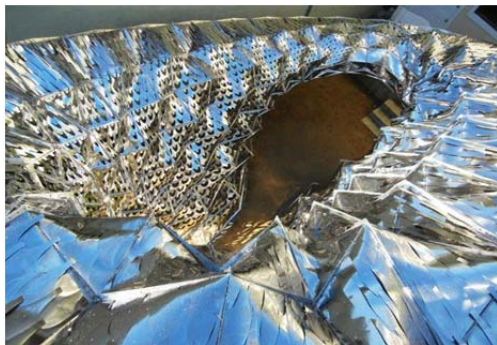
Fig. 8: Metal Mesh reacting to heat
